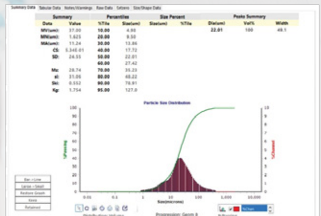
Fig. 7: LD particle size report from SYNC, including percentiles, summary statistics data and frequency / cumulative distribution graphs
