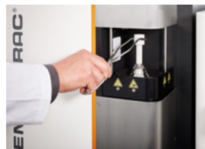
Placing sample with accelerator on the pedestal of the ELEMENTRAC CS-i
