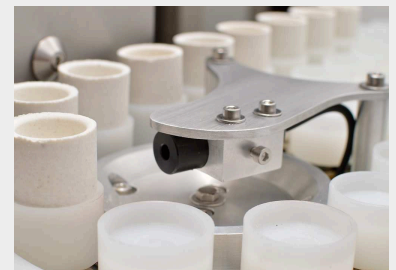
Autoloader with acid-resistant plastic crucible holders
