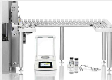
Autoloader with 130 crucible positions
