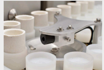
Autoloader with acid-resistant plastic crucible holders
