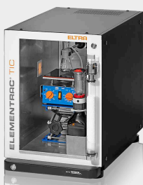
Analyzer with optional TIC module
