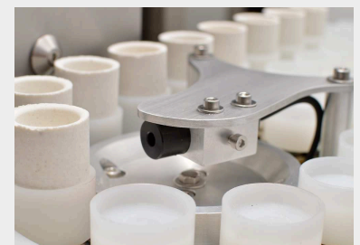
Autoloader with acid-resistant plastic crucible holders
